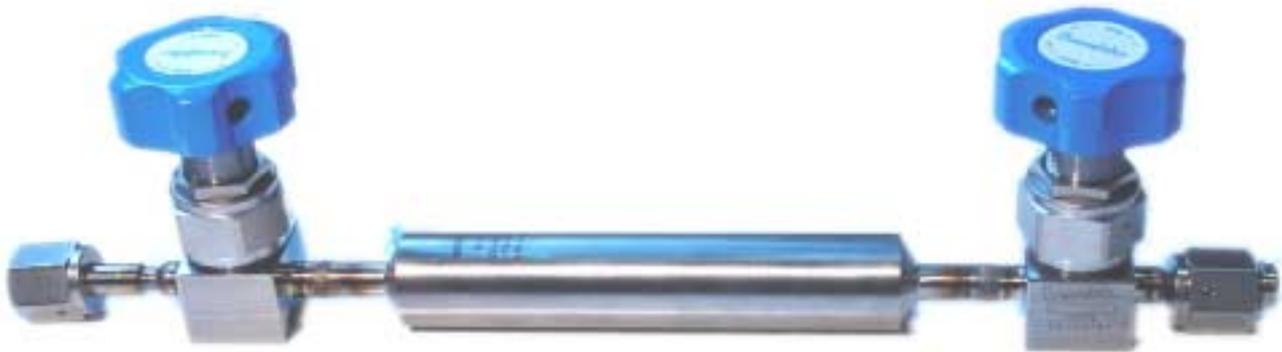
**CAUTION** : COLLECTION CYLINDERS ARE SHIPPED TO YOU UNDER VACUUM. DO NOT OPEN VALVES UNTIL READY TO COLLECT SAMPLE. AFTER SAMPLE HAS BEEN COLLECTED, BE SURE TO CLOSE VALVES BY FINGER TIGHTENING ONLY.
